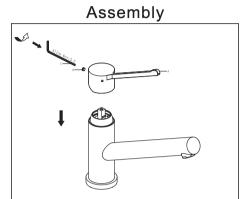
Disassembly: Using a 2.5mm allen key (C) to loosen grub screw (D) and remove handle (E). Assembly: Fit new handle (A), taking care that it is pushed fully onto cartridge stem, and use a 2.5mm allen key (C) to lock the grub screw (B) tightly.
